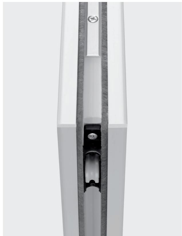
By exchanging the duoPort S bogies, the bearing capacity can be increased from 70 kg to up to 140 kg.
