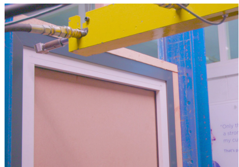
Mechanical loading test
