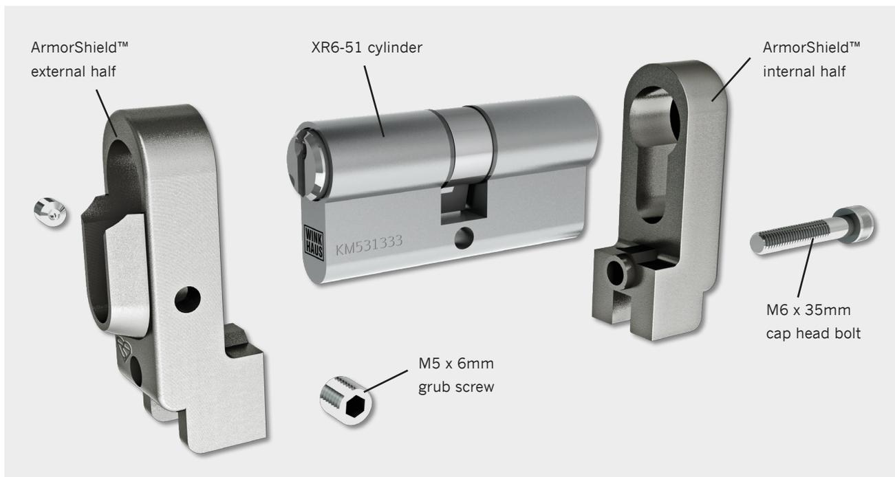
Exploded view of ArmorShield™ and XR6-51 Kitemark cylinder (TS007 3☆ Combination). M6 bolt is used to hold the ArmorShield™ halves together and 2 grub screws are tightened to help prevent the cylinder being removed if a 'snapping' attempt is made
