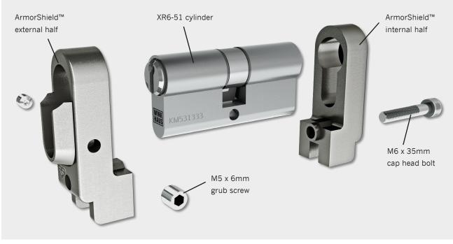
Exploded view of ArmorShield<sup>™</sup> and XR6-51 Kitemark cylinder (TS007 3☆ Combination). M6 bolt is used to hold the Armorshield<sup>™</sup> halves together and 2 grub screws are tightened to help prevent the cylinder being removed if a 'snapping' attempt is made
