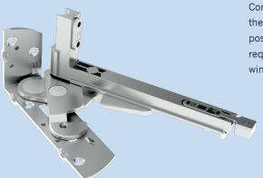
Complex technology on a small footprint: Excellent air gap tolerance due to the low stack height of the corner frame and sash hinge. 3D adjustment is possible without any special tools. The additional sash support bar is only required for sashes exceeding 100kg reducing the cost of the majority of windows produced.
